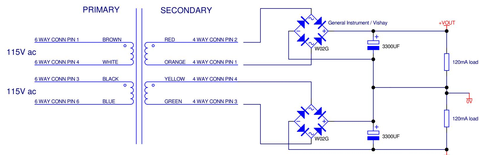
Pin-outs of Molex connectors, as viewed looking down at the end the wires enter the connector
